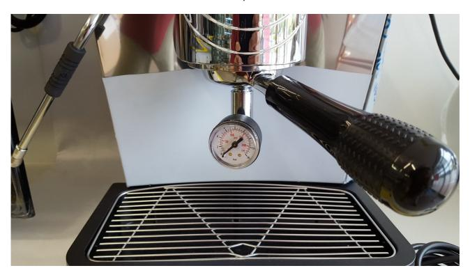
Press the button to dispense coffee, the manometer will read an X pressure To **DECREASE** the pressure unscrew anticlockwise the adjustment screw of the OPV valve
